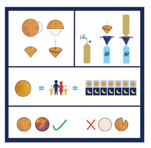
water for a family. Filters are used with Keystone Funnel ™ for simple hands-free water filtration using any common household water container.
