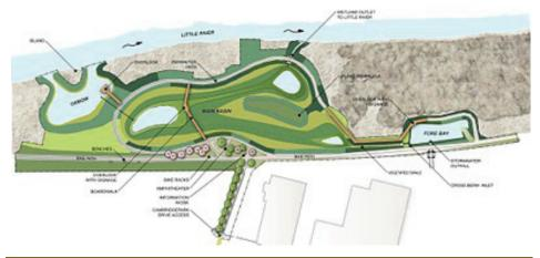
**Cambridge Stormwater Wetland System** Earthen levees and spillway structures interface with trails, boardwalks, overlooks, an amphitheater, native plants, and wetlands.
